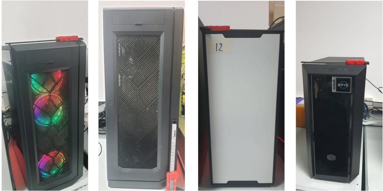
Figure 2 The four Cloud servers. Three on the left are dual-socket Intel Xeon with a number total core of 36-48 cores. The server on the right is a dual-socket 48-core AMD EPYC. The servers are accessed remotely by several users.
