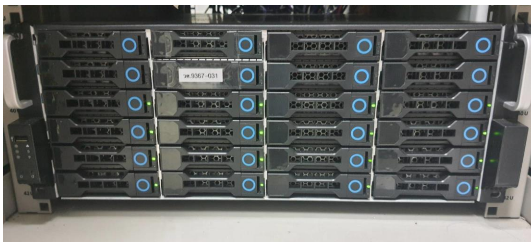
Figure 4 Disk storage server of the APPLY cluster with 308 TB total capacity.
